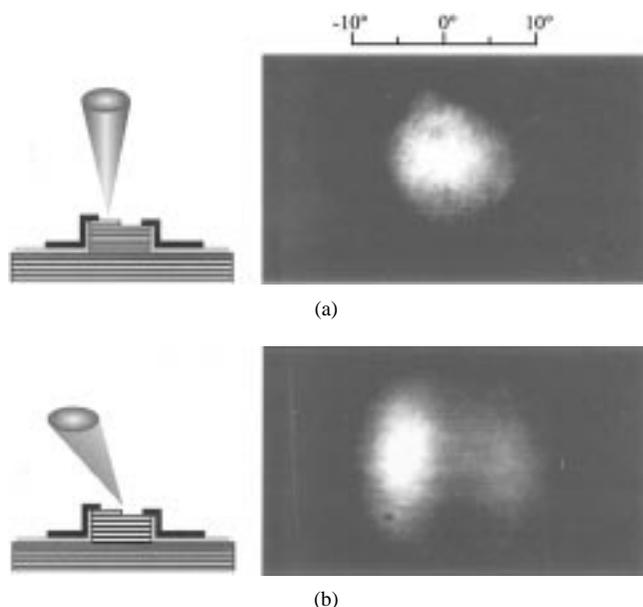
Fig. 2. Far-field patterns of the beam-switching VCSEL when current is injecting to (a) only the nonphase-shifted area; (b) both areas.
