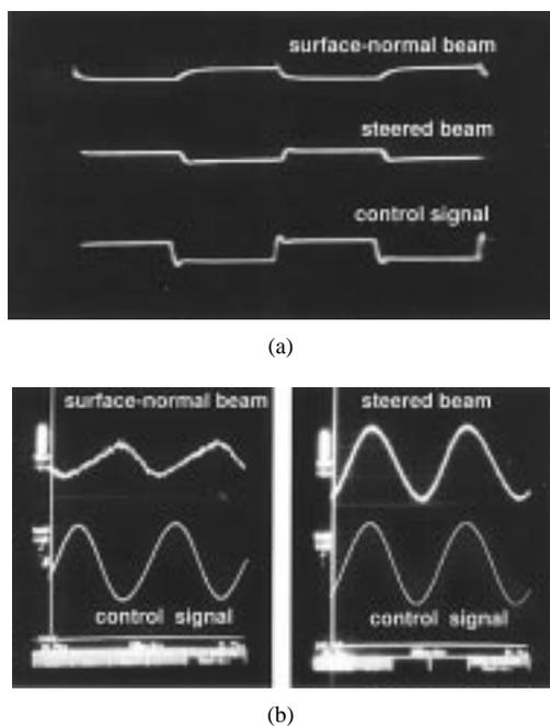
Fig. 3. Dynamic beam switching of the VCSEL when the phase-shifted area is modulated by a control signal at (a) 1 MHz and (b) 2 GHz. The surface-normal beam and the steered beam are separated by a spatial filter.
